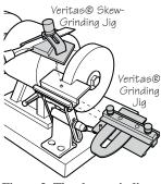
Figure 3: The skew-grinding jig and grinding jig.
