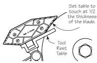
Figure 6: Setting the tool rest angle.
