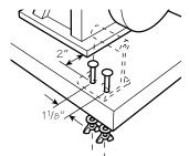
Figure 2: Mounting hole locations.
